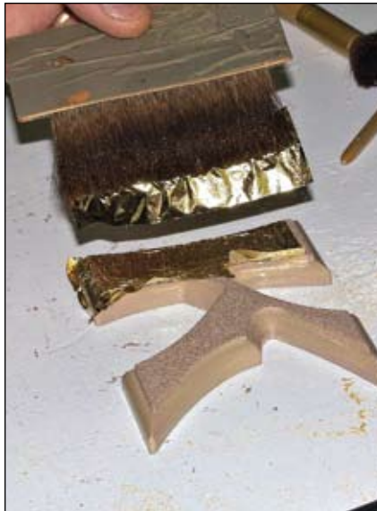
When doing a sand gild I find that you must factor and bid the work as if you are gilding twice as it will take twice the amount of gold to cover all the bumps and moguls of the sand surface. The gold leaf is laid and then pressed firmly into the size with a foam brush.
