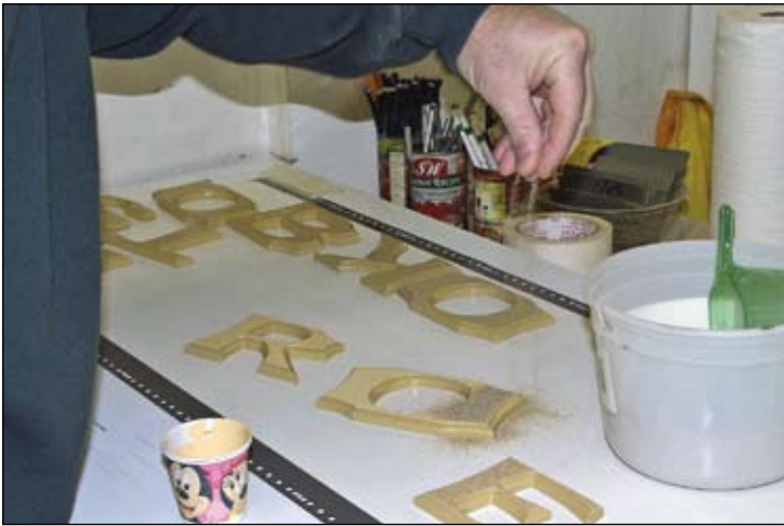
The letters were primed and then finished with 1 Shot lettering enamel and allowed to dry. The faces were given a second coat and while still wet fine sand (like table salt) was sprinkled over the entire surface and allowed to completely dry. Once dry the loose sand was poured off and the letters were cleaned with a brush and compressed air.
