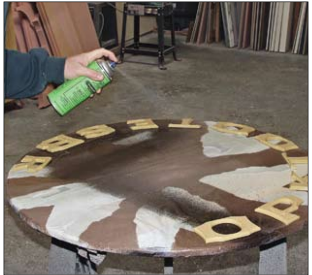
I suggest sealing the sand prior to sizing for gold leaf. Frog Juice in the aerosol can is a quick way to accomplish this step.
