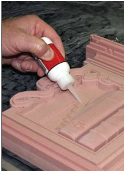
Strength to weight ratio is very high with cyanoacrylate so you don't need to use too much glue. The book is lightly sprayed with the accelerator and then applied to the receiving pad and becomes permanent within three seconds.
