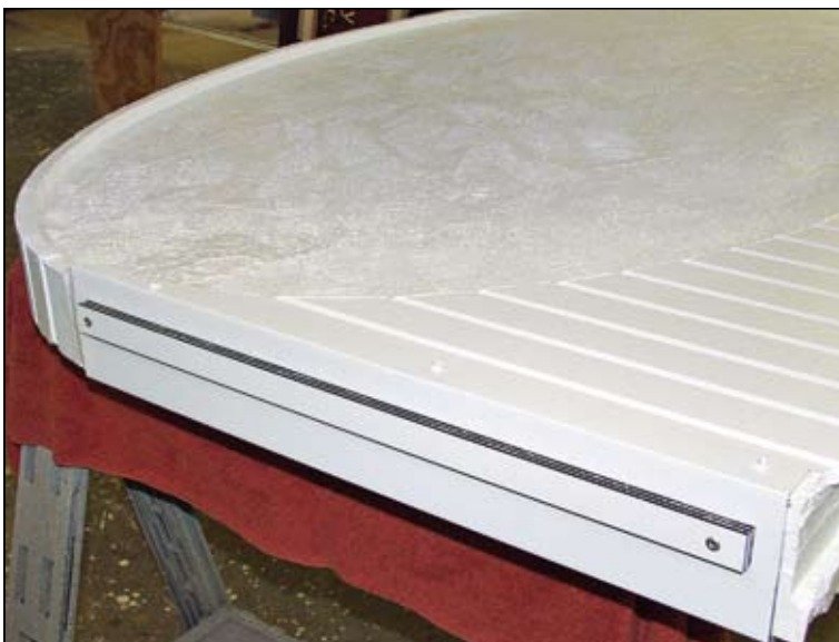
Because of budget restrictions one of the old signs was treated as a redo but it had the same rotten center core as the sign that got broken. We had to rebuild the ends to be able to have strength when secured into the dado of the posts. To fix the problem we cut Dibond and through bolted it on the ends.
