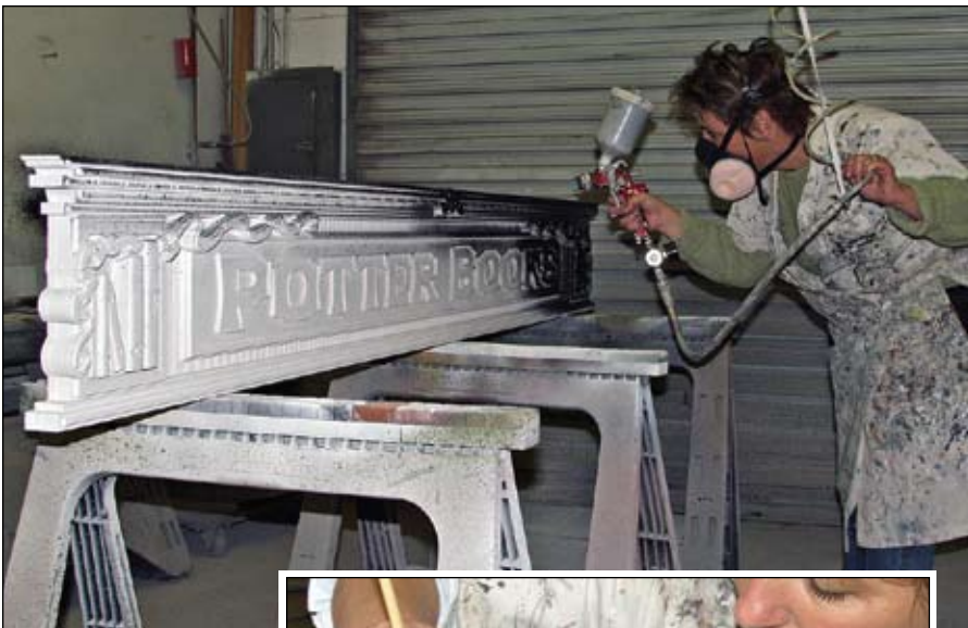
Normally we will spray the primer coat and finish coat using the HVLP spray gun but because this sign was so small we elected to brush the primer by hand to get into all of the small areas. The black finish coat (100% acrylic) was sprayed and while still wet Robin came back and worked the paint into the deep crevices.
