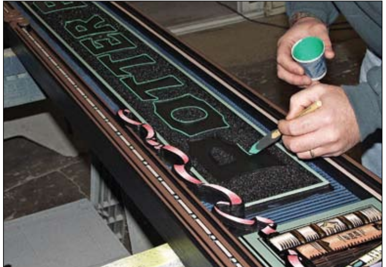
After dumping the excess smaltz onto a large piece of pattern paper and returning it to the master container I was able to paint the green letter outlines.
