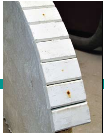
After a decade of service the signs were showing their age. The MDF back panel had completely disintegrated and the metal hardware like the nails around the border were showing the rust.
