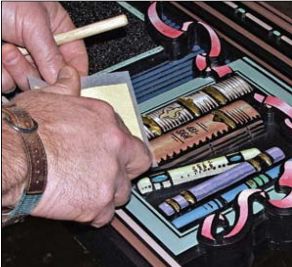
The gold bands on the bookbindings were sized and gilded using patent gold leaf.
