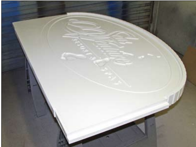
The new sign was cut on the Gerber router, primed then finished with acrylic paint.
