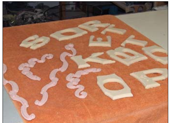
The ribbons and letters are cut separately from the main sign. The ribbons will be attached to the sign before any priming takes place. As with the decorative moldings the ribbons were cut separately to allow for easier tooling with the router.
