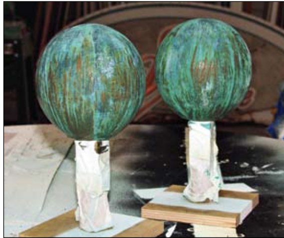
The finials were treated with three coats of Modern Options copper surfacing paint. While the last coat is still wet I sprayed the finials with the patina green solution to achieve a nice natural patina color.
