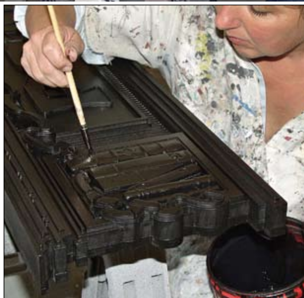
Normally we will spray the primer coat and finish coat using the HVLP spray gun but because this sign was so small we elected to brush the primer by hand to get into all of the small areas. The black finish coat (100% acrylic) was sprayed and while still wet Robin came back and worked the paint into the deep crevices.
