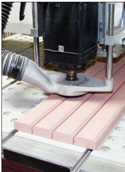
I used the router to cut the planks that surround the border of the sign. The planks were cut to length and bonded to the border with cyanoacrylate glue. For consistent placement and overhang I used the jig shown here (with arrow).
