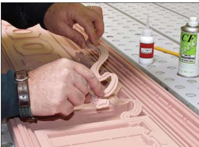
The ribbons are permanently glued to the sign using cyanoacrylate glue and an accelerator. This glue is ideal for use with high-density urethane and the immediate bond is a real time saver.
