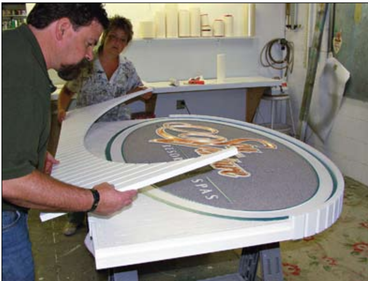
Silicone adhesive is applied to the sign and the skirts are carefully positioned in place.
