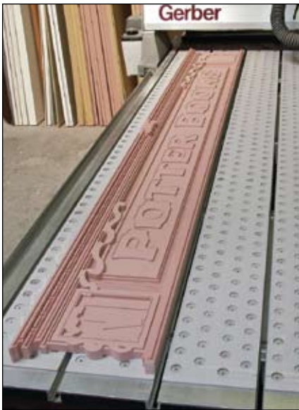
10-lb. Signfoam 3 with a 1" thickness was cut on the Gerber router. Fitting the bits into the small areas was the most difficult part of this sign. Otherwise the design is a bunch of rectangles requiring cleaned out areas.
