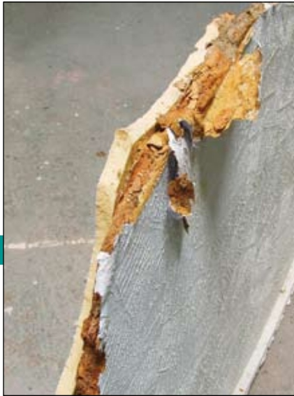
After a decade of service the signs were showing their age. The MDF back panel had completely disintegrated and the metal hardware like the nails around the border were showing the rust.
