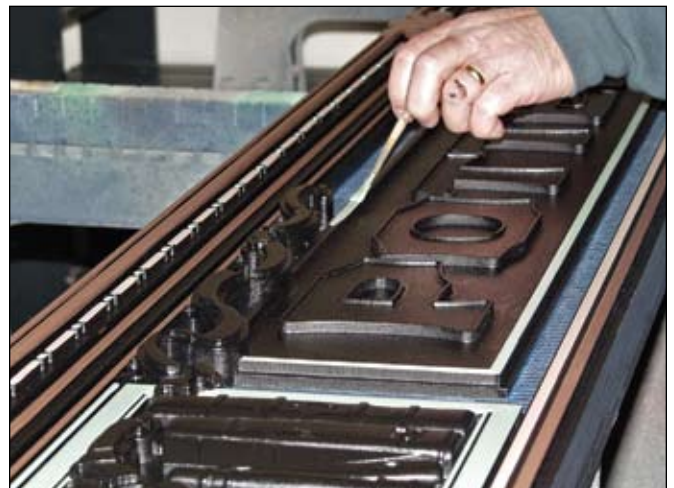
All color is painted with 100% acrylics. The only low lying area to paint was the blue background area. Otherwise all areas were on top. Using a red sable bound in a quill I sweep on the color keeping the brush handle at a very low angle to the surface. Working in this manner achieves a heavier film of paint on the surface and keeps run-over to a minimum.
