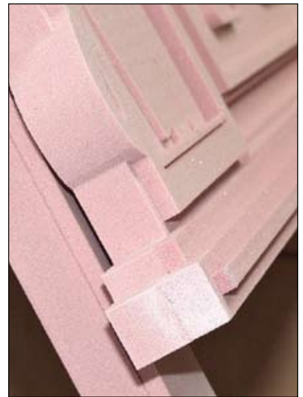
The decorative moldings at the top and bottom of the sign were cut separately and glued permanently to the sign with cyanoacrylate glue. This allowed me to manage the appearance of thickness and also made for easier tooling with the router.
