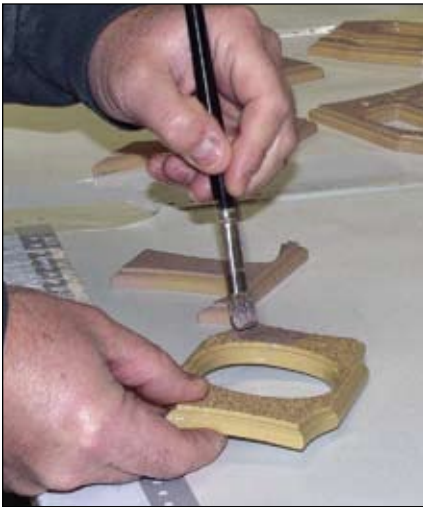
To create plenty of open time for a "gild ready" letter, 1 Shot quick size and Lefranc 12-hour size are mixed in equal parts and applied to the entire letter. In my particular atmospheric conditions the size was ready for gold within four to five hours.
