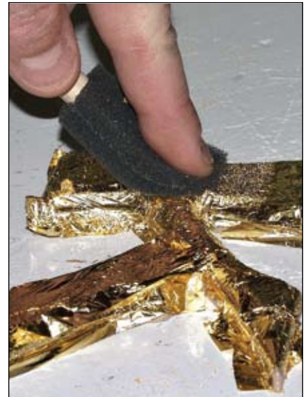
When doing a sand gild I find that you must factor and bid the work as if you are gilding twice as it will take twice the amount of gold to cover all the bumps and moguls of the sand surface. The gold leaf is laid and then pressed firmly into the size with a foam brush.
